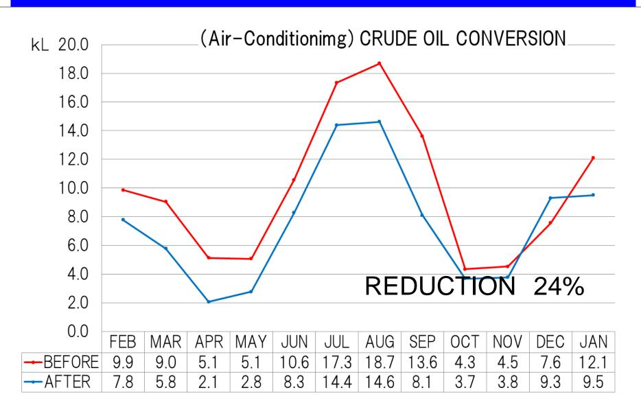
The main purpose of the liquid desiccant processor is to help improve the IAQ, however, its by-product is high energy efficiency of 20 to 70%, depending on the amount of ventilation.
