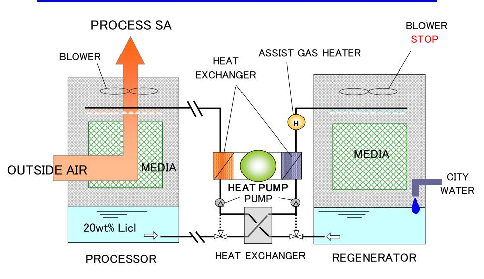
Please take a look at this slide. This slide shows the schematic of a standard liquid desiccant processor operating in the humidification mode in mid-winter.
