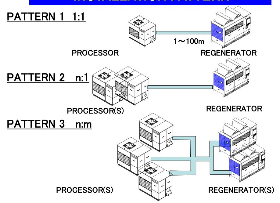
The processor is comprised of a pair of units, the OA processor and the solution regenerator. We have several variations as you can see in the Power Point slide. They can be installed right next to each other, or as far as 100 meters apart, practically.
